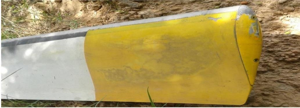
**Photographs showing exposed bond line on the blade (without debonding)**
