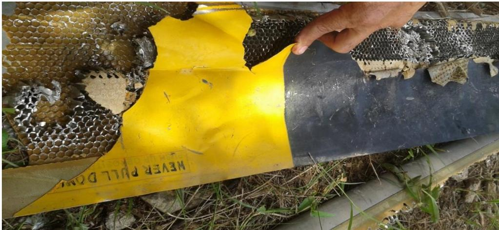
**Photographs showing peeling of the blade skin with consequential damage to honey comb structure**
