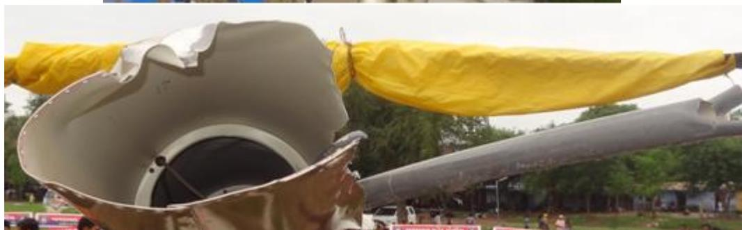
**Photographs showing separation of tail rotor boom from the rivets**
